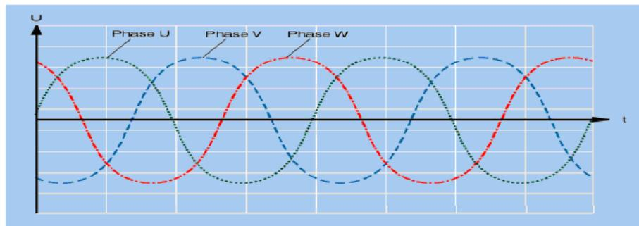
A perfect symmetrical sine wave supply; the sum of three phases is equal to zero
