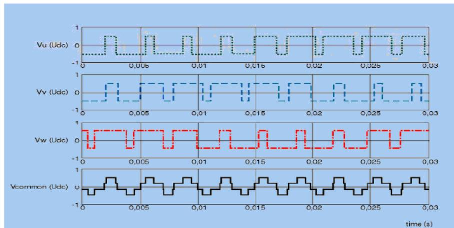
Common mode voltage; the sum of converter output phases is not equal to zero
