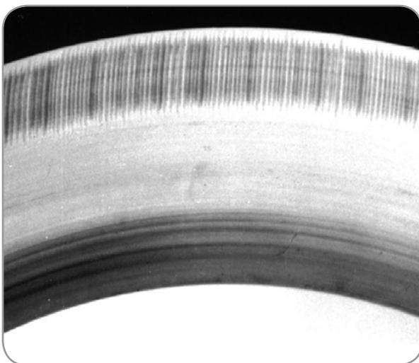
Figure 7: Fluting on the outer ring raceway of a bearing
