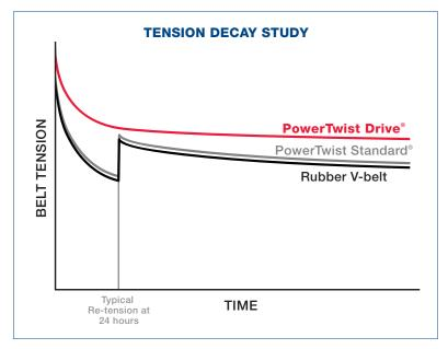
Extensive testing was conducted to track the tension decay of PowerTwist Drive versus PowerTwist Standard and a comparable rubber V-belt. Test results show that PowerTwist Drive maintained the required tension throughout the duration of the test. PowerTwist Standard and rubber V-belts require re-tensioning to maintain proper belt tension.
